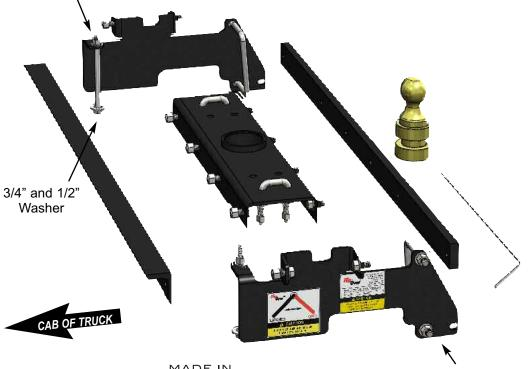
Model Number 238 Gross Trailer Weight: 30M lbs. Gross Trailer Tongue Weight: 7.5M lbs. Use forward hole for most trucks, rear hole with wider u-bolts if truck has Firestone air bags.
